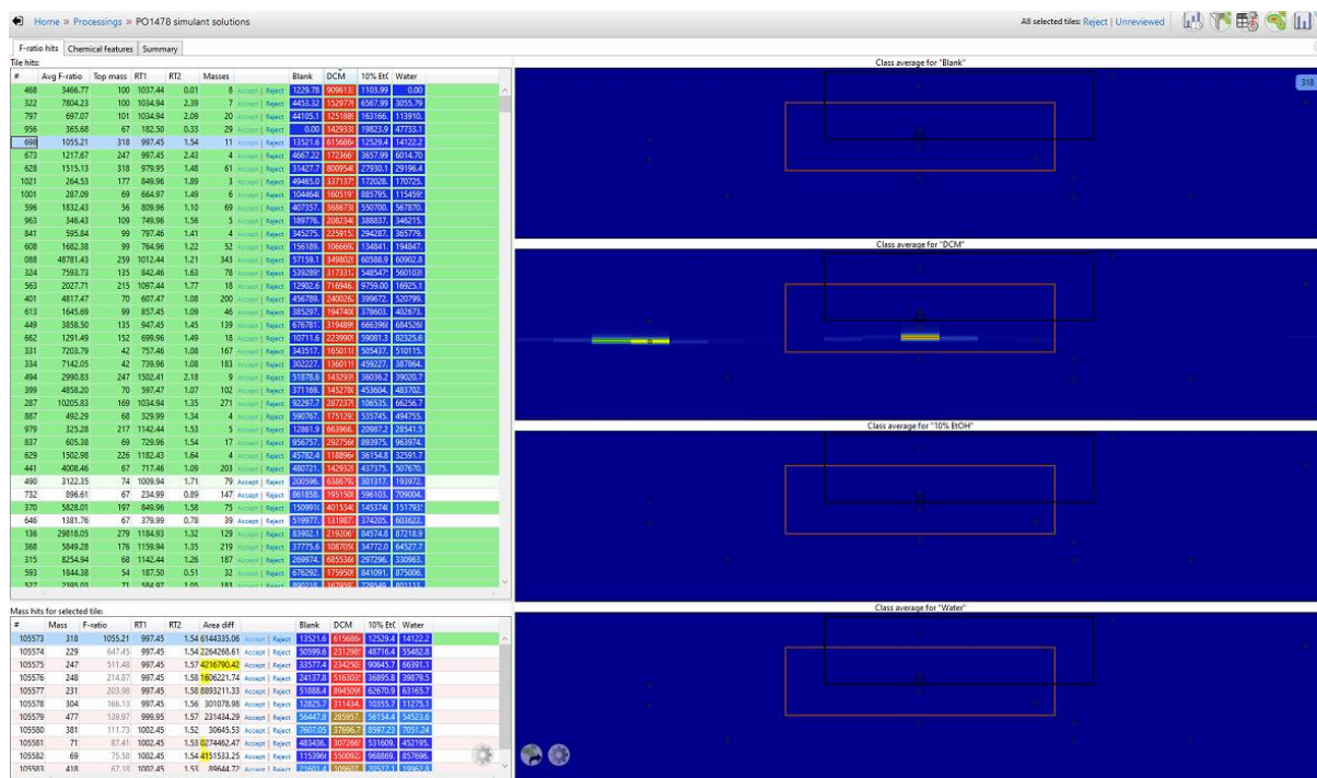
Figure 3: Initial F-ratio analysis showing list of features with associated F-ratio and masses found for each sample class (left). Feature intensities are also depicted with heat maps, red being most intense. The contour plots to the right show a selected feature within a tile (red box) for each sample class.
