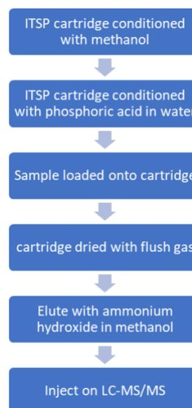
Figure 2: Automated procedure for sample extraction and analysis.
