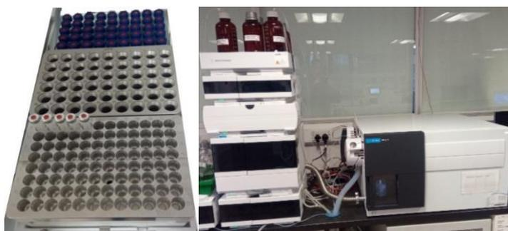
Figure 1: ITSP setup and Agilent 1200 LC with 6470 MS/MS
