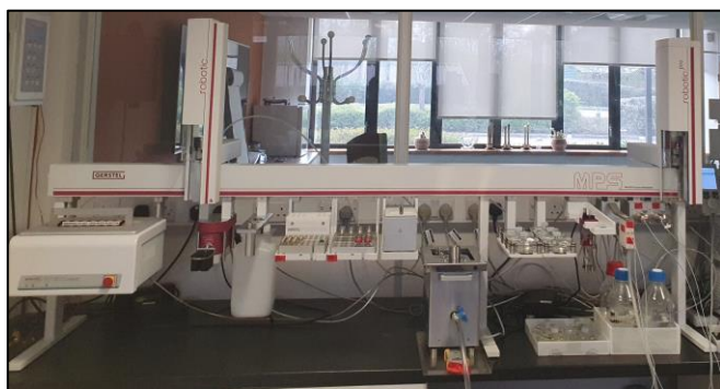
Figure 2: Automated sample prep configuration for the analysis of nitrosamines in selected drug substances Link to video
