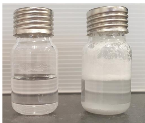
Figure 4: Example of drug substance preparation for Metformin and Irbesartan after mixing, sonication and centrifugation
