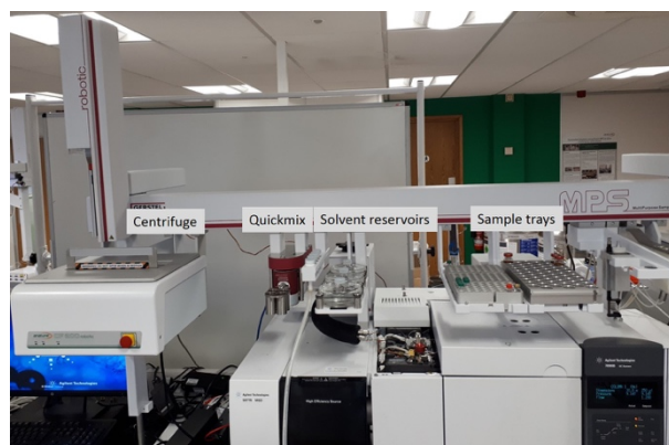
Figure 2: Fully automated DiLLME solution.
