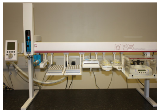
Figure 2 – Gerstel MPS for automated immunosuppressant extraction.
