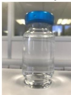
The picture on the left depicts a 10mL high recovery vial which enables the recovery of small amounts of solvent.
