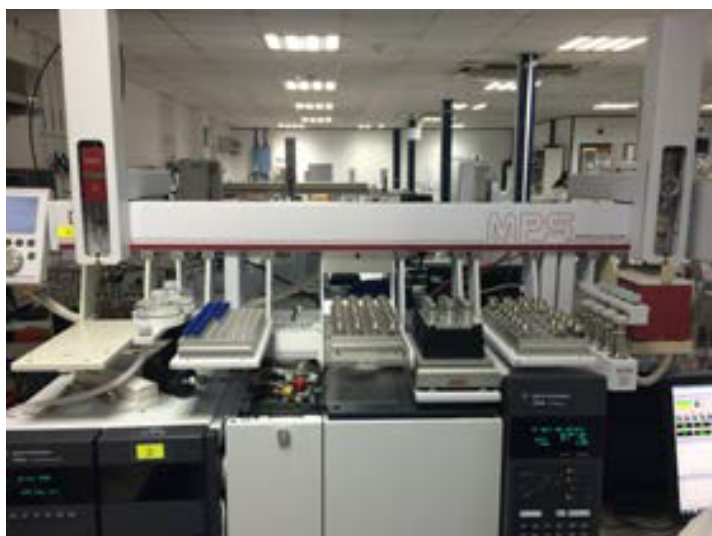
Figure 1: GERSTEL Dual Head MPS XT with Agilent 5977B
