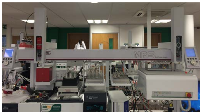
Figure 2 GERSTEL Dual Head, mVortex and Centrifuge with Agilent GC-MS (5977) at Anatune
