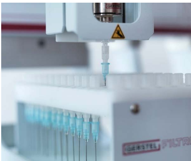
Figure 3. Pictures of the MPS transporting the 0.45 \mu\text{m} filter from the filtration tray (left) to the VT-98 tray with filtration cover (right).
