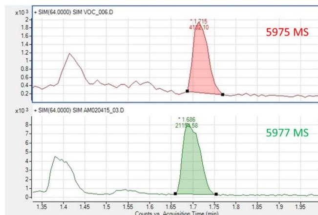
**Figure 4: SIM chromatogram comparison between an Agilent MS 5975 and 5977 for bromomethane and chloroethane at 0.5 µg/l**
