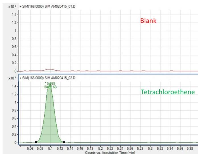
Figure 3: SIM chromatogram (ion 166) comparison of a blank and tetrachloroethene at 0.1  $\mu\text{g/l}$
