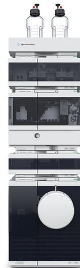
The Agilent LC/MSD (liquid chromatograph/mass selective detector) achieves sensitivity and resolution specifications with autotune.
